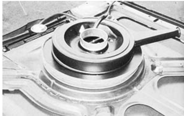
Another angle from underneath showing spacer, air cleaner, ring and seal flush against bottom of cowl induction hood.
