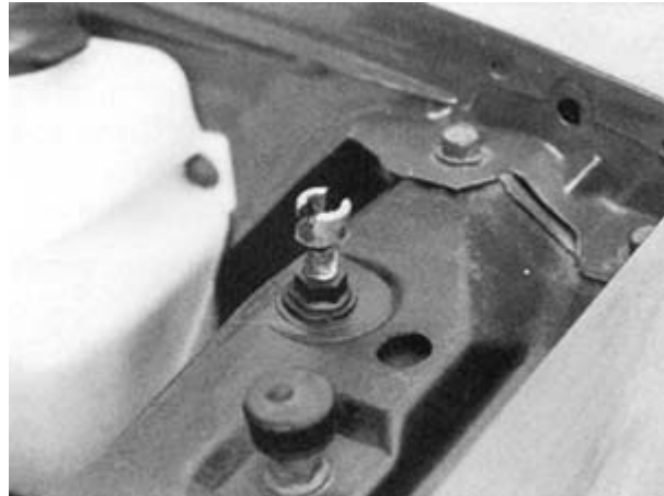
Radiator support has dimpled area for hood pin studs. The support must be drilled to install studs. This photo shows accessory hood locking pin stud. Note correct style nut.
