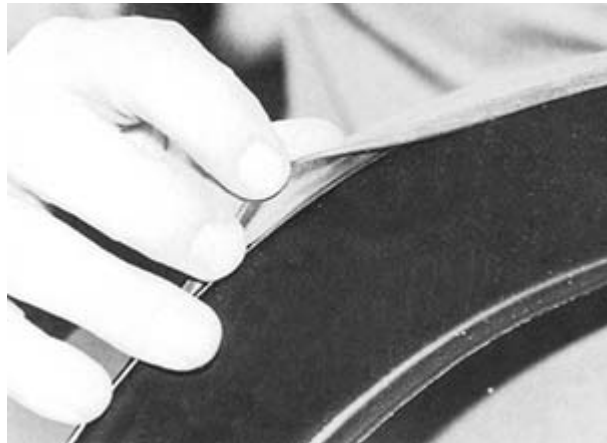
Start at any point to install seal on flange. Seal joint should be located at back on centerline of engine. Black adhesive can be used for installation, but is not necessary.
