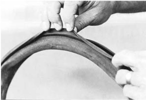
Air cleaner flange seal has lip that slides over ring.
