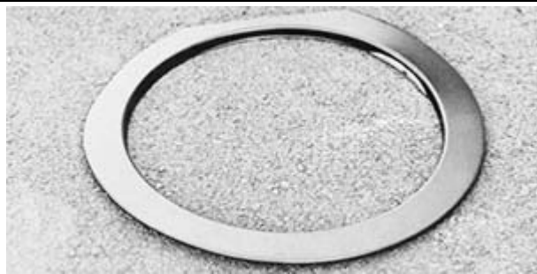
Cowl induction ring flange holds rubber seal. Flat side of ring faces RH side. Lip on ring flange sits down into the air cleaner base.
