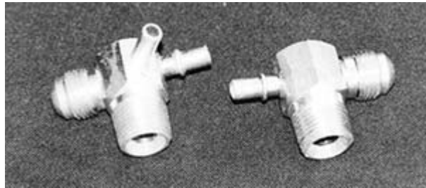
Vacuum fitting is located on back of intake manifold between carburetor and distributor. Metal booster brake line is on left and 18 inch hose to flow valve is on right.
