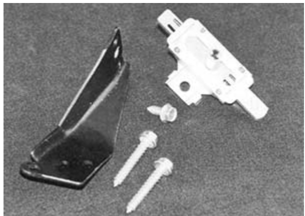
Kick down bracket and gas pedal switch. This unit operates the electrical components of the hood and activates the Turbo 400 passing gear for cars equipped with automatic transmission.
