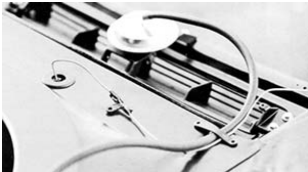
Wiring harness is taped to plastic retainer. Hose and wire are strapped to bottom side of hood.
