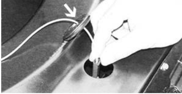
Cowl induction wiring harness for solenoid should be threaded through hood grommet.
