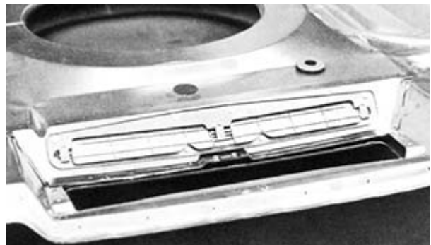
Six bolts with star washers are used to attach air valve assembly to hood.
