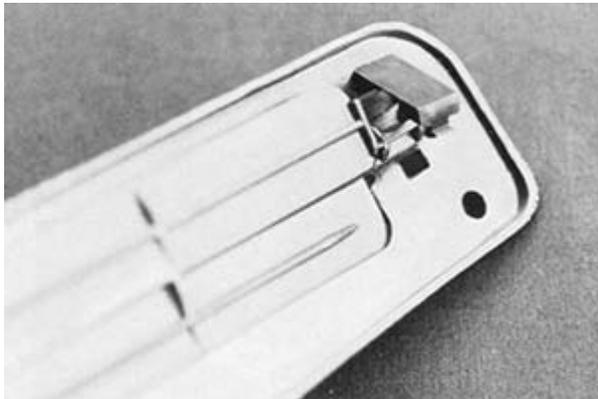
*Shorter side of air valve overlaps frame that faces rearward. Air valve clips snap into slots.*
