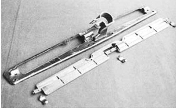
*Air valve frame, air valve door and three attaching clips. Wide side of air valve overlaps frame assembly on solenoid side of frame.*
