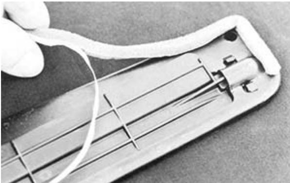
*Foam seal for frame assembly has adhesive tape on one side. Material molds easily to conform around perimeter of frame. Notice chip tabs in slots of frame and wider side of air valve.*
