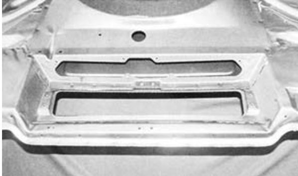
*Bottom side of bare cowl induction hood. The opening closest to edge of hood is for outer flapper door. Second opening is for inner door or air valve assembly.*
